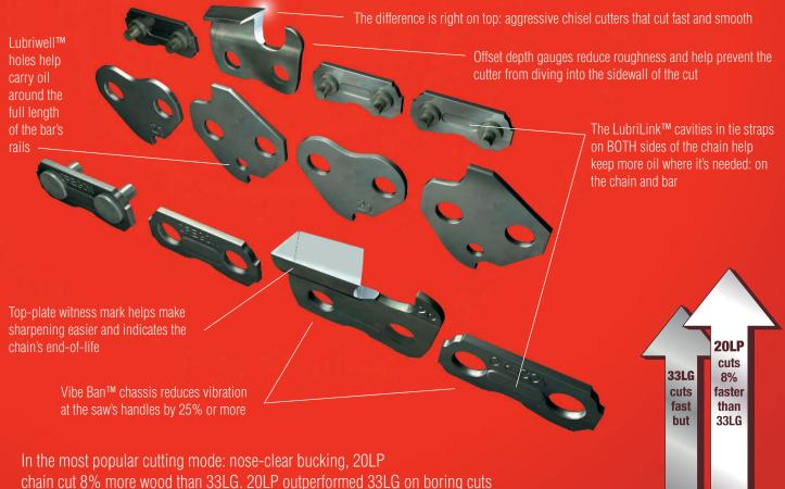
and bias cuts as well. Test wood used: Douglas Fir, test saw used: Husgvarna 340 with a 16" bar.
